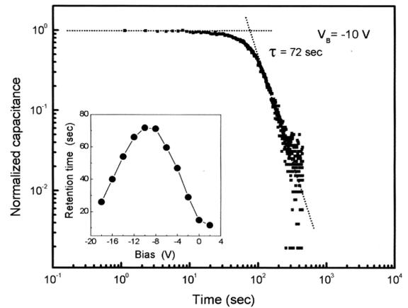
Fig. 4.  $C$ - $t$  characteristics of IBAED sample at -10 V after injecting electrons at 20 V for 8 sec. The inset shows the retention time variation as a function of bias voltage.
