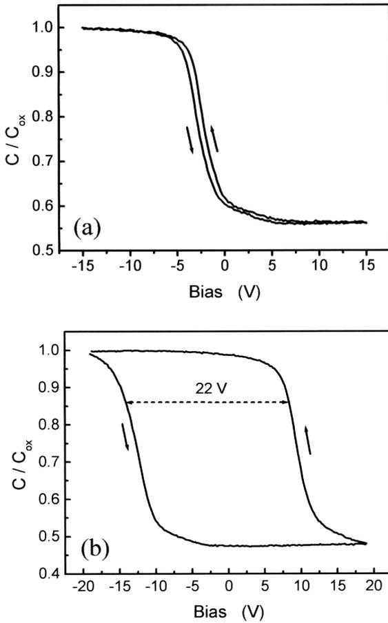
Fig. 1.  $C-V$  characteristics of EBD sample (a) and IBAED sample (b). A dual sweeping mode is employed for  $C-V$  characteristics. Arrows in the figures are sweeping directions. Sweeping rate is 2 V/s.
