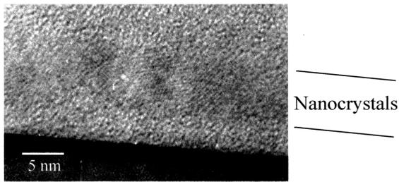
Fig. 3. Cross-sectional TEM image of IBAED sample RTO-treated at 1000 °C.
