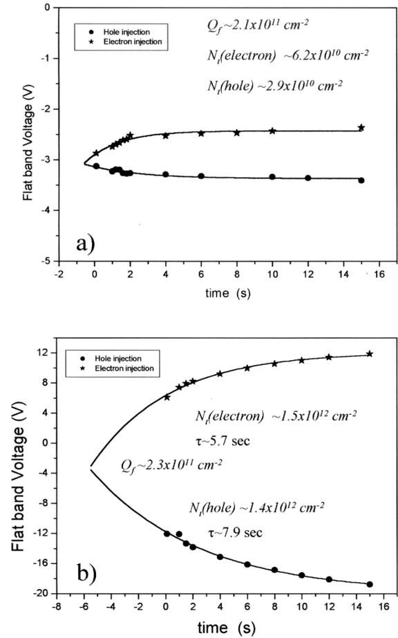
Fig. 2. Flat band voltage shift as a function of injection time of EBD sample (a) and IBAED sample (b). Electrons/holes are injected at +20V/-20V and sweeping rate during measurement is 20 V/s.
